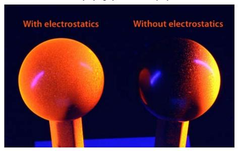
Take a look at these two ceramic test targets. Each spray was the same except for one thing – the left target was sprayed with the electrostatic charging system ON, but the right target was sprayed with the charging system OFF. The results are *astounding*.
